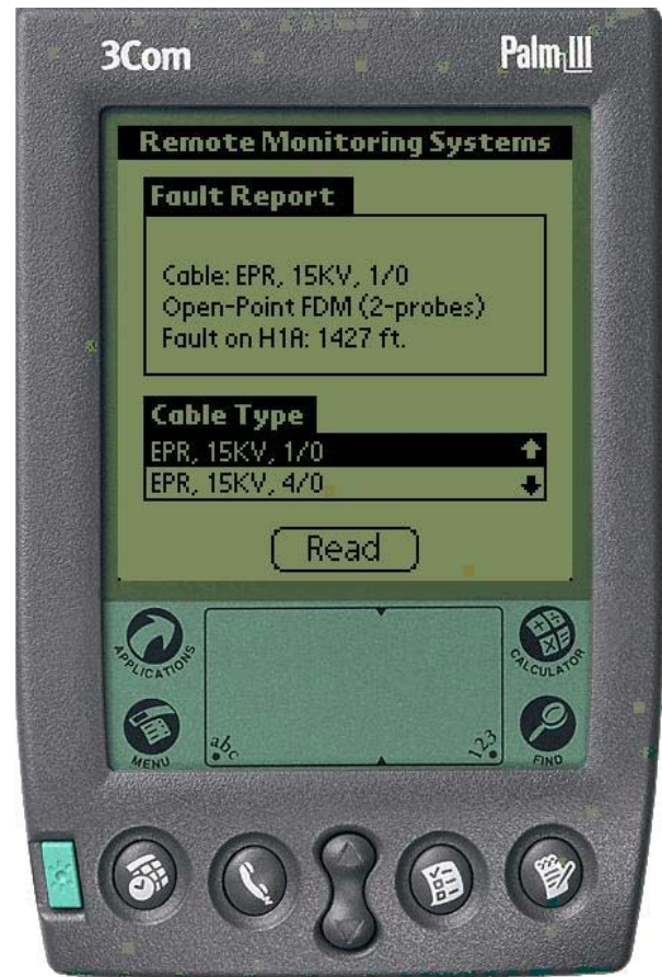
Figure 3. BeamIt™ Fault Distance Monitor Report
